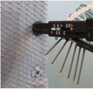
Auto-feed screw guns with magnetic nose cup adaptor to rapidly attach insulation and lath into heavy gauge steel studs.
