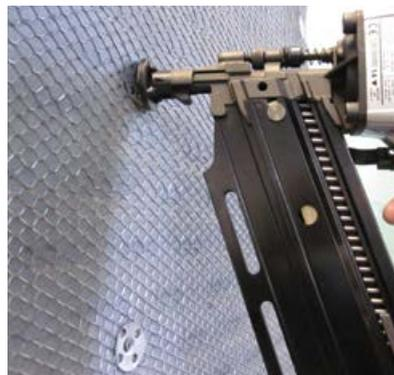
Pneumatic guns with custom magnetic nose cup adaptor to rapidly attach insulation and lath into wood studs.
